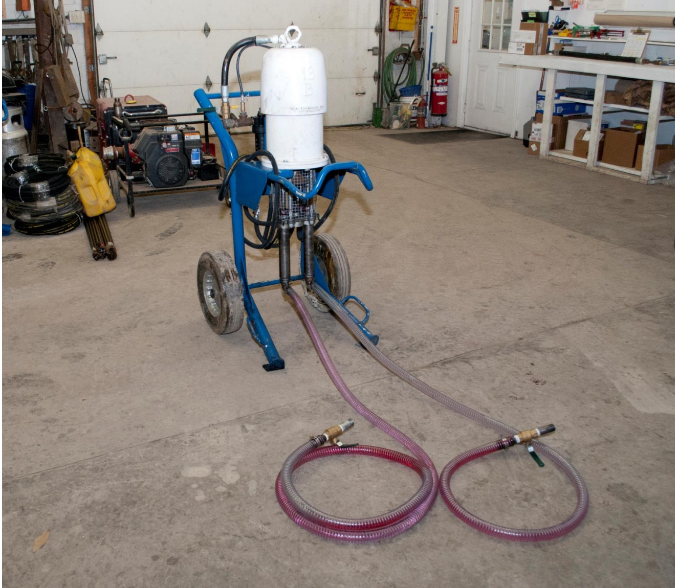
Air Pump set up. This example is set up to pump dual component formulations at up to 5500 psi
